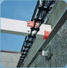
GRP return rails with wear shoes
